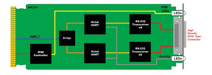
FIGURE 1. AMC301 Functional Block Diagram
